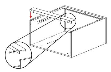
**7.** Place the rear flange of the bottom (Ref. No. 9) into the bottom lances of the back. The flange with two holes should face the front, hanging over the sill. Insert bolts through the bottom and sill with the head facing the front of the unit.
