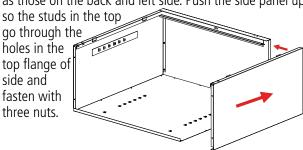
**6.** Attach the sill (Ref. No. 6) to the sides. Place nuts loosely on each of the studs and slide the ends of the sill into the slots on both sides of the unit. Then, securely tighten the nuts.
