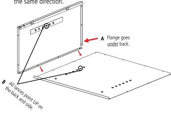
**4.** Attach the top (Ref. No. 5) to the unit by sliding the outer flange over the back of the unit and the side flange to the side panel on the unit. The threaded studs should go
