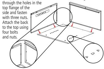
**5.** Attach the right side (Ref. No. 3) to the back in the same manner as you did in step 3, again making sure that the flange is around the back and that the lances on the shelf adjustment strips are pointed in the same direction as those on the back and left side. Push the side panel up so the studs in the top
