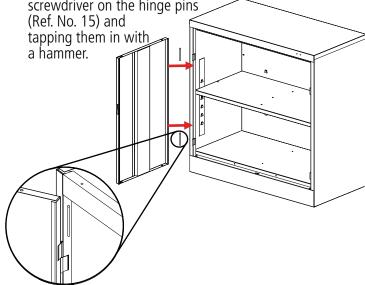
**11.** Attach the right door (Ref. No. 8) to the unit in the same way you attached the left door.
