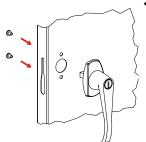
1. Place the locking handle (Ref. No. 11) on the right hand door and fasten with two #8-32 X 1/4 hex-head bolts and lock washers, provided with the handle.
