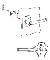
With the handle still in the open position, hook the locking bars (Ref. No. 10) to the locking cam (see "A" at left). Once in position, slowly rotate the door handle to the closed position so the lock bars prot rude from the holes at the top and bottom of the door (shown at right, below).
