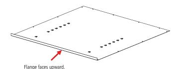
**3.** Attach the left side (Ref. No. 2) to the back by placing flange (A) around the back and bolting the back and side together with four bolts and nuts (Ref. Nos. 17 & 18). Be sure that the lances on all shelf adjustment strips (B) point in the same direction.
